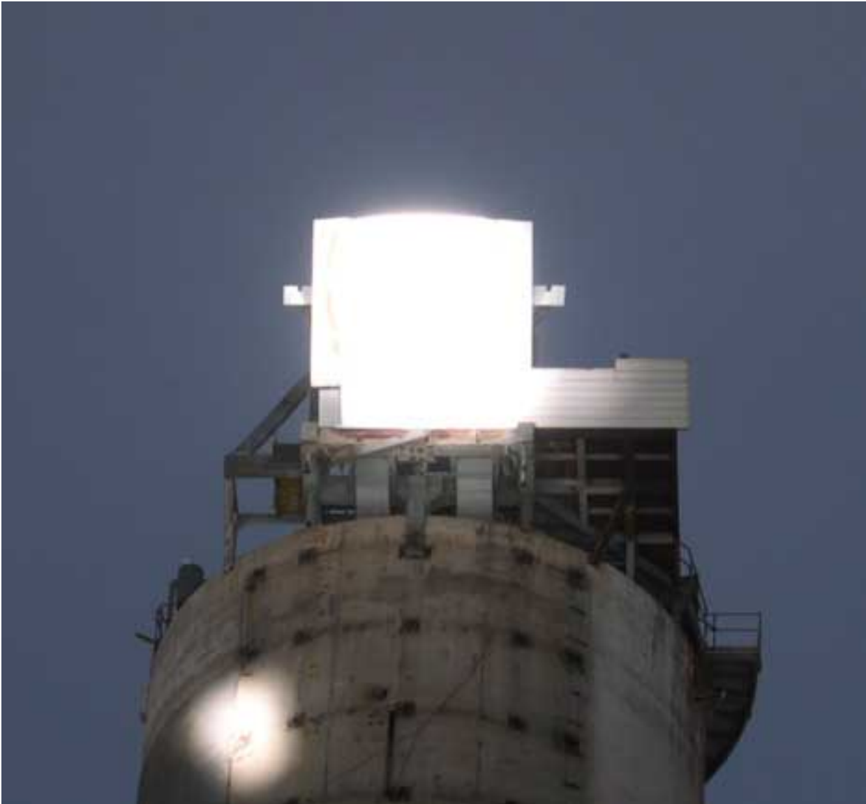
The final testing of 270 pcs ceramic VR-units from the SolAir project spring year 2004.
