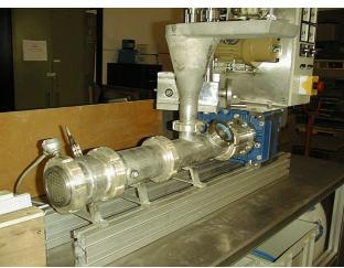
We even build commercially operating multi-cell re-crystalized Silicon Carbide extruders for Dines and CeraMem.
