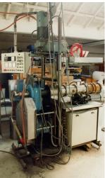
Besides the extruders we designed and manufactured many Extrusion Die Heads, Air Beds, Rotating dryers, Cutting devices, Capping equipment, Coating apparatuses, furnaces, test equipment – all for manufacturing of multi-cell re-crystalized Silicon Carbide honeycombs.
