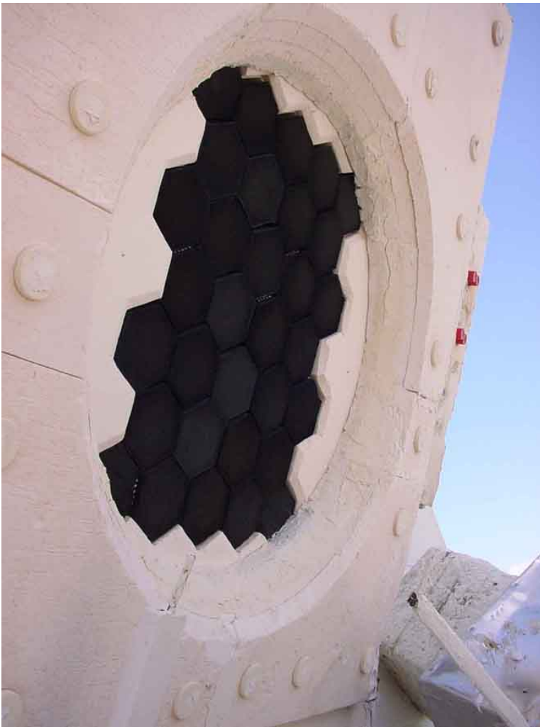
HitRec2 close up fall 2000 on the tower with the 36 VR units being encapsulated in alumina insulation boards
