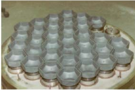
Fig. 5: HitRec I stainless steel construction
