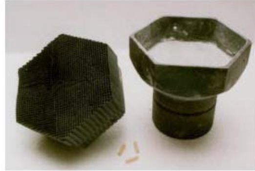
Fig. 6: HitRec I absorber module, monolith and cup
