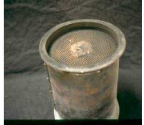
This is the actual Corning WFF tested on a Bukh diesel engine at DTU in 1986, which started the extensive development work for a more robust WFF
