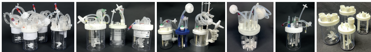
Various mini-SUBs with as low as 50 ml Working-Volume in a 150 ml Vessel Volume SUB. Several sizes which adapt to any PCS brand in the market most often with Magnetic-Bottom-Drive on a Magnetic-Stirrer-Table (MST) from CerCell adapting to any servo motor. Off course with pre-installed Single-Use-Sensors (SUS) as needed.
